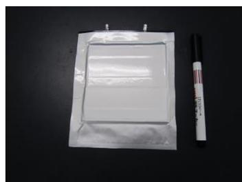
secondary lithium polymer battery secondary batteries
