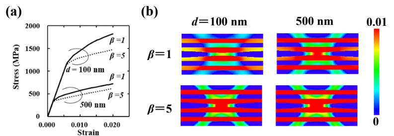
Fig. 2 (a) Stress-strain curves of ferrite phase with different layer thicknesses  $d$  and dislocation absorption abilities  $\beta$  and (b) distributions of equivalent plastic strain in  $(\theta/\alpha/\theta/\alpha/\theta/\alpha/\theta)$  lamellar structures when tensile strain is 1.7 %.
