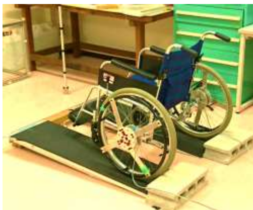
Fig.1 Wheelchair with 6-DOF force sensor
