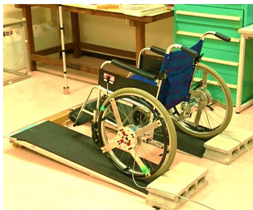
Fig.1 Wheelchair with 6-DOF force sensor
