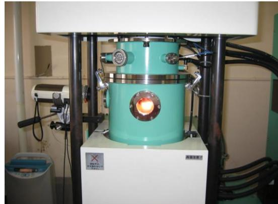
Photo. Pulse Electric Current Sintering at 1500°C
