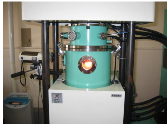
Photo. Pulse Electric Current Sintering at 1500°C
