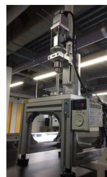
Friction measuring device for soft material ring
