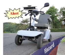
Fig.1 Hazardous Object Detection System
