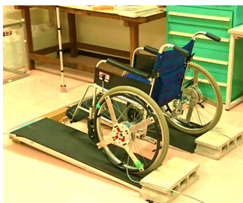
Fig.1 Wheelchair with 6-DOF force sensor
