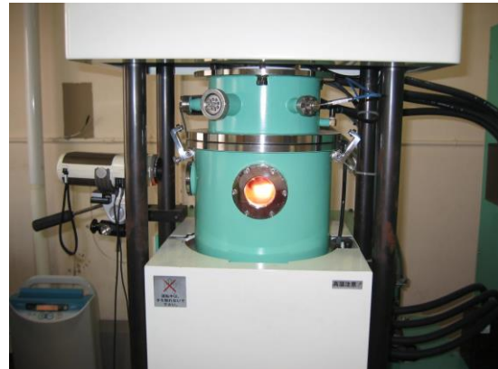
Photo. Pulse Electric Current Sintering at 1500°C
